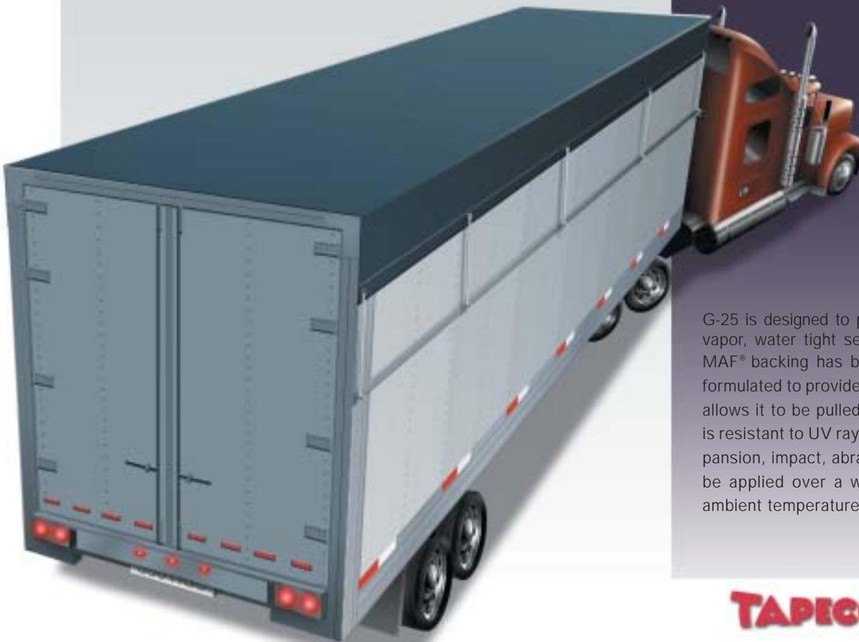
G-25 is designed to provide an air, vapor, water tight seal. Its unique MAF® backing has been specially formulated to provide strength that allows it to be pulled tightly. G-25 is resistant to UV rays, thermal expansion, impact, abrasion and can be applied over a wide range of ambient temperatures.
